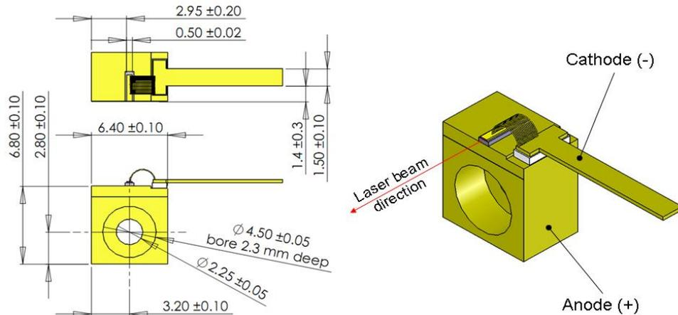
The C-mount is an ideal component for quick prototyping and laboratory setups. However, the maximum output power is typically limited by the sub-optimal heat dissipation properties of the C-mount itself. Please contact us to discuss the best package option for your application.
